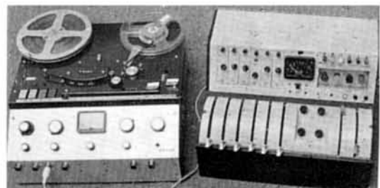
Fig. 7 Tape Recorder Developments recorder and the author's stereo mixer used in the music tests.
