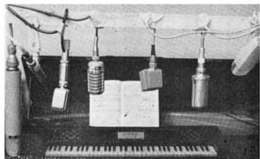
Fig. 6 The five microphones under examination, a Reslo, and the author's capacitor design, suspended above a Mozart piano.
