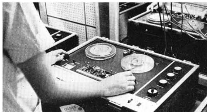
Above: The main Sony plant at Shinagawa, Tokyo. Below: A TC530 undergoing final listening tests.
