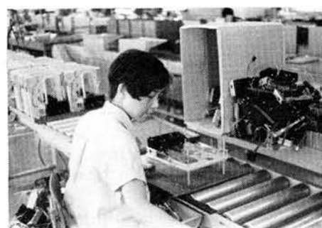
Early stage in assembly of the X-4 battery recorder
