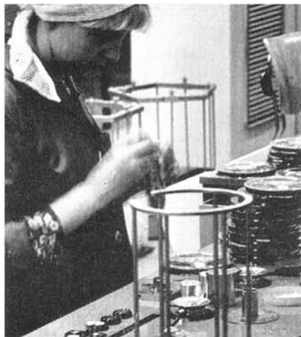
Final stage of production. The tape is wound on to branded plastic spools.
