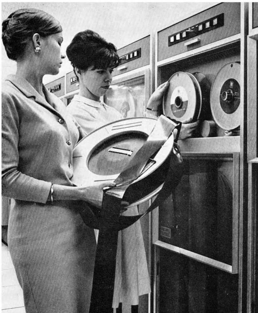
The computer is sometimes accused of rendering human labour obsolete. An irony is visible in this photograph, which shows a giant tape reel from a Honeywell Datamatic computer —itself made redundant by the newly-installed H-800-111 in the background.
