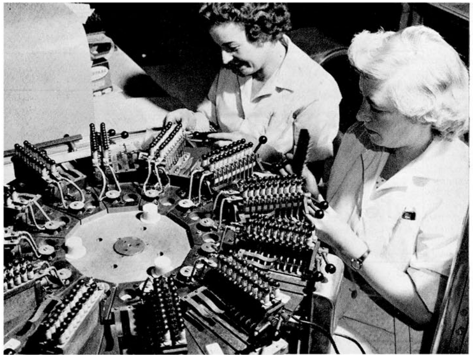
Fig. 4 (upper left): Germanium power transistor assembly line.
