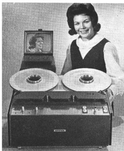
Above: Ampex VR303 fixed-head video recorder employing \frac{1}{2} in. tape. Left: Large and small cases containing Sony video recorder and camera kit.
