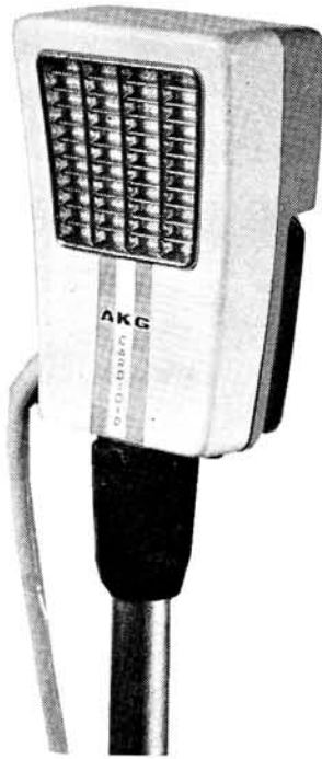
Left: Res/0 figure-of-eight ribbon microphone; note grille at front and rear of ribbon housing. Right: AKG moving-coil cardioid microphone.
