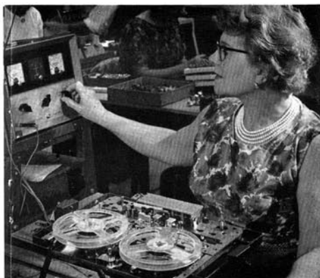
Below : Speed fluctuations being measured on a Gaumont Kalee flutter-meter.
