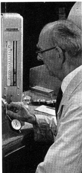
Below : Speed fluctuations being measured on a Gaumont Kalee flutter-meter.
