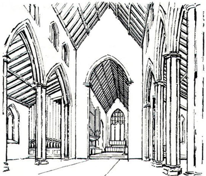
Fig. 2: A church such as the one shown here may suffer from an unbalanced organ effect, part of the instrument speaking out into the Chancel but with important sections of it speaking out Westwards into the Nave.
