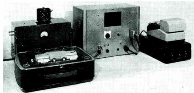
Fig. 17: A dropout-counting equipment used for routine production testing. Left-hand unit contains circuitry as in fig. 14, centre unit is the counter and timing control for the printer, right. The clock works with the timing unit and rings to warn operator at end of set period. (Photo by permission of M.S.S. Recording Co. Ltd.)
