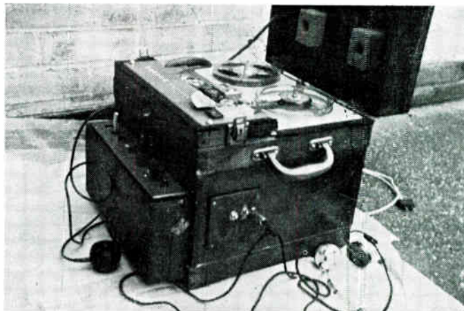
The extra head is situated by the off key, and the tape is not threaded for transistor playback to show the guide.
