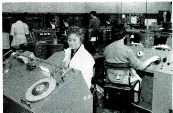
Fig. 5—The re-spooling machine (seen in operation in the foreground of the illustration) provides automatic inspection of the coating by a photo-electric system. In the background can be seen the machines for "pen-testing" Emitape.
