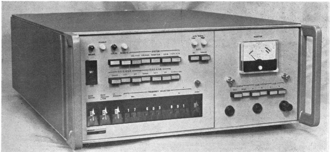
General appearance of the new Marconi H2900 receiver, covering 1.5 to 30 MHz, with a tuning accuracy to one cycle (1 Hz). The read-out as set in this picture shows that the Rx is tuned to a frequency of 17,603 kHz and 891 cycles (Hz). The applications of the H2900, a highly sophisticated design, are mainly military and commercial. In size it is only 22 x 17½ x 7in. high, and its weight is 91 lb.
