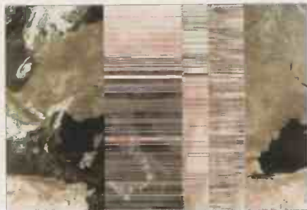
Fig. 1: NOAA-16 image 1223 21 September showing sync fault.
