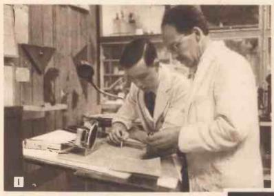
I. Engineers and draughtsmen devise the layout for the "Little Maestro," created at Pilot Radio's factory at Park Royal, Acton. When the lay-out is finished laboratory samples are passed, Bills of Material prepared and component parts released
