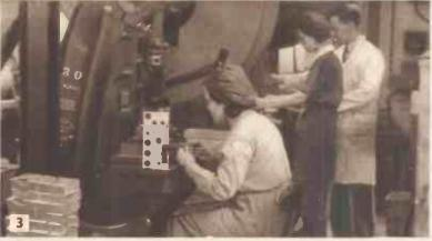
3. The next operation takes place on the Stamping Press, where in one rapid movement the blank steel is shaped as a chassis and all the necessary holes for the valve holders, gang condenser and tuning controls are stamped out. The chassis is then cadmium plated
