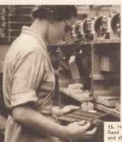
15. Now the back is fixed on the receiver, and the number of the chassis recorded for reference
