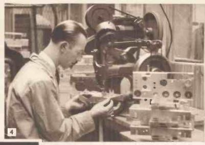
4. Leaving the Tool Room the chassis is transported to the riveting assembly. This photograph shows an operator fixing valve holders, drive spindle and other brackets necessary for mounting such components as the electrolytic and gang condenser
