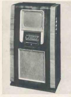
Philips Television 1939/40 Type 2415 de luxe model of the new range gives a big picture measuring 10 ins. by 8 ins. Incorporating a 5-valve all-wave receiver, it has the Philips Automatic Tuning and many other refinements
