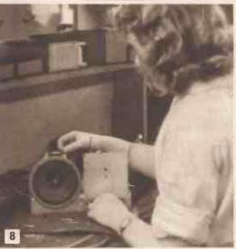
8. The operator is seen adding the speaker to the chassis, which is connected to its high tension and signal supply, the 25Z6 valve. The long and medium wave coil is also fixed on the chassis and wired through
