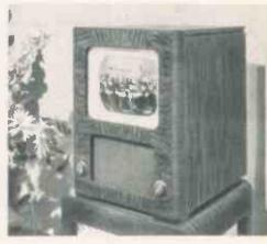
This H.M.V. Television Model 1800 is a complete table model receiver giving an 8% ins. by 6% ins. picture. It includes a noise-suppresser on both sound and vision, so it can be used where motor car interference is likely to be heavy
