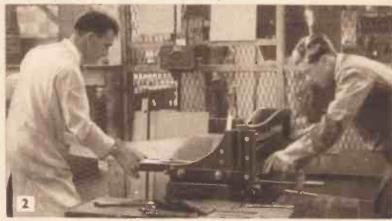
2. Component parts which have to be purchased from outside suppliers are thoroughly checked to the finest degree of accuracy. This picture shows blank sheets of matal being cut to the required size by guillotines, which are very sharp blades worked by leverage
