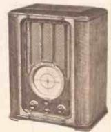
MODEL U.355, 5-Valve Superhet for A.C. Mains. Three wavebands 16-52, 180-540, 800-2,000 metres. 5½-inch Compass Dial. Fast and Slow tuning. 8-inch Speaker. 3 watts undistorted output.
