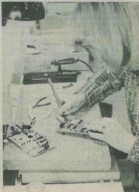
In this assembly station at Oxford Medical Systems the operator builds the complete product. Components are brought forward as required by a Link-Hampson "Trescomp" motorised conveyor.
