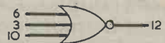
Fig. 5. The interconnections illustrated in this circuit allow the 4007 to function as a 3-input NOR gate.
