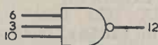
Fig. 6. Another configuration for the multi-option 4007. This time it operates as a 3-input NAND gate.
