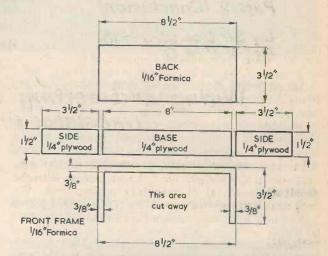
Fig.7. A suitable case for the receiver may be made up with the items shown here.
