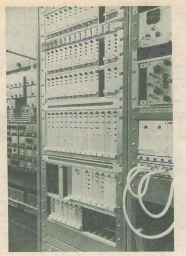
A close-up of one of the bays of equipment in the BBC p.c.m. system. (Courtesy BBC).
