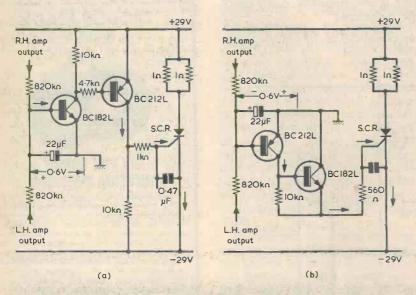
Fig.5(a). If the non-earthy terminal of the  $22\mu$ F reservoir capacitor is taken about 0.6 volt positive of chassis the upper two transistors turn on and trigger the thyristor. The arrows show current flow (assumed to be from positive to negative).
