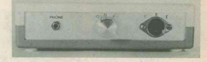
The Go-No Go Transistor Tester. The only control is the 3-way switch in the centre of the front panel, and this selects "Off", "N.P.N." and "P.N.P." The test transistor connects to the DIN socket on the right of the panel.
