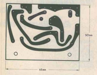
Fig. 2. The layout of the amplifier is rather critical. A suitable printed circuit board is shown here, reproduced full size.
