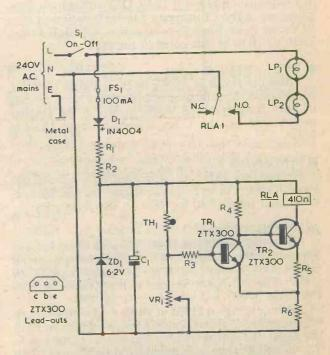
Fig.1. The circuit of the airing cupboard warmer. Thermistor TH1 is the temperature sensor, and the lamps are controlled by the contacts of relay RLA.
