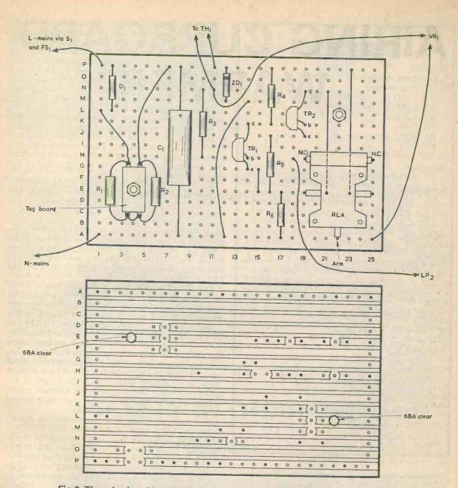
Fig.2. The relay is soldered directly to the Veroboard panel, as also are most of the other components. Veropins suitable for 0.15in. Veroboard are employed at the connection points to parts external to the board. Fig.1 should be followed for circuit details not shown here.
