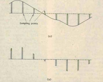
Fig. 1(a). The amplitude of an analogue signal is sampled at regular intervals. (b). Each sampling operation produces a pulse whose amplitude is equal to the amplitude of the analogue signal at the time of sampling. This is a pulse amplitude modulation version of the analogue signal.
