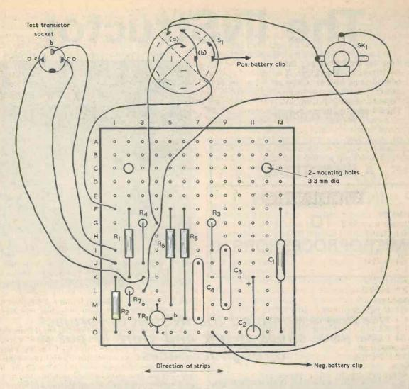
Fig.3. Wiring up the transistor tester. There are no breaks in the copper strips of the Veroboard. Before wiring to S1(a) (b) confirm the corresponding inner and outer tags with a continuity tester in case the switch employed has a different tag layout to that shown here.
