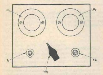
Fig.3. Apart from the thermistor and the lamps, the components are all enclosed in a metal case. The two lampholders, S1, VR1 and the fuseholder are fitted to the top panel.
