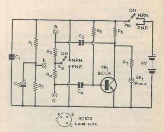
Fig.2. The circuit of the Go-No Go Transistor Tester. The transistor under test connects to the points indicated as "E", "B" and "C". The transistor tester with its top cover removed. A phone jack socket different to the more common "open" type shown in Fig.3 was used in the prototype.
