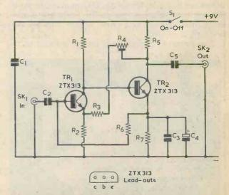
Fig. 1. The circuit of the a.c. coupled 20dB amplifier. Both transistors are high speed devices, giving a bandwidth extending to at least 20MHz.
