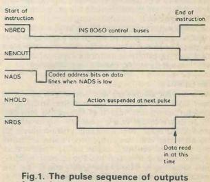
from the 8060. This shows only command pulses, not the address pulses nor any data outputs. The accumulator is, as its name suggests, the main store of the microprocessor, where all numbers that are to be operated on are loaded into or taken from. How do we know that this number is loaded in? We can check by asking the microprocessor to "write" it out again, but we'll need to see what has to be done to write data out first.
