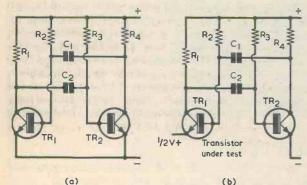
Fig.1(a). Basic astable multivibrator with n.p.n. transistors.
