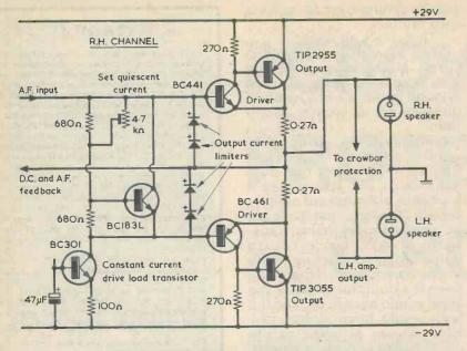
Fig.2. The driver and output transistors of the right hand channel amplifier appear in the circuit shown here, with connection to the right hand speaker being made via a DIN socket. The left hand amplifier stages are identical.
