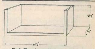
Fig.8. The pieces of Fig.7 made up to form the case, into which the receiver assembly slides. The dimensions shown here and in Fig.7 are for guidance only, and the case should be made, in practice, to take the receiver assembly as constructed.
