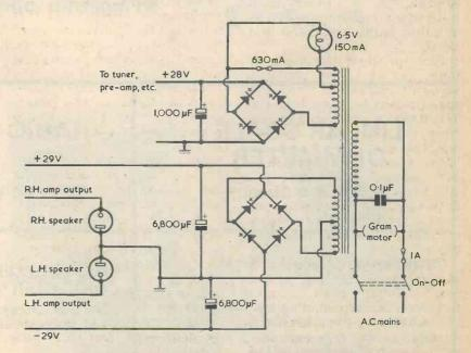
Fig.1. Power supply circuit in the hi-fi unit serviced by Dick. The two 29 volt rails supply the right and left hand power output amplifiers. The pilot lamp connects to a 6 volt tap in the upper mains transformer secondary. There was no continuity: the fuse had blown. Dick studied the service manual once again.
