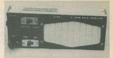
The assembled receiver in its home-constructed case.
