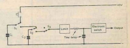
Fig.1. Simplified circuit illustrating the sequential operation required in S1 and S2, and the time delay components between the latch and electronic switching sections of the combination lock.
