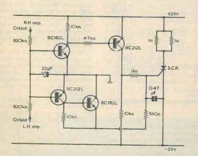
Fig.4. The crowbar protection circuit. The two  $1\Omega$ resistors in parallel limit the short-circuit current which flows when the silicon controlled rectifier, or thyristor, is fired. This circuit, and those of Figs.1 and 2, are slightly simplified versions of the corresponding circuits in the Ferguson 3987 Hi-Fi Unit.
