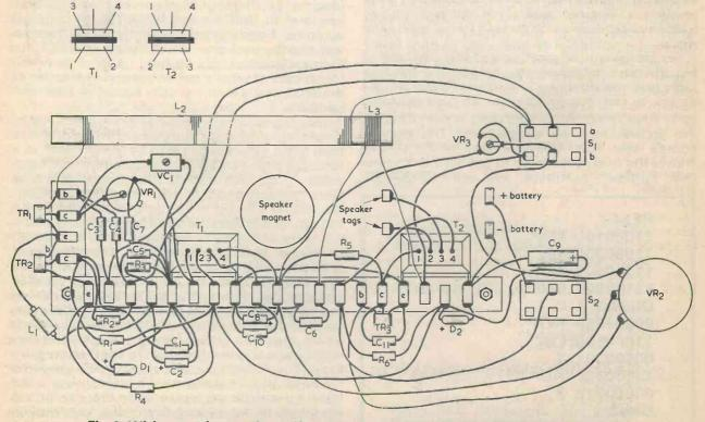
Fig.6. Wiring up the receiver. The cathode end of zener diode D2 is indicated by a plus sign. Components are shown spread out for clarity but in practice should be kept within the outside edges of the receiver front panel.
