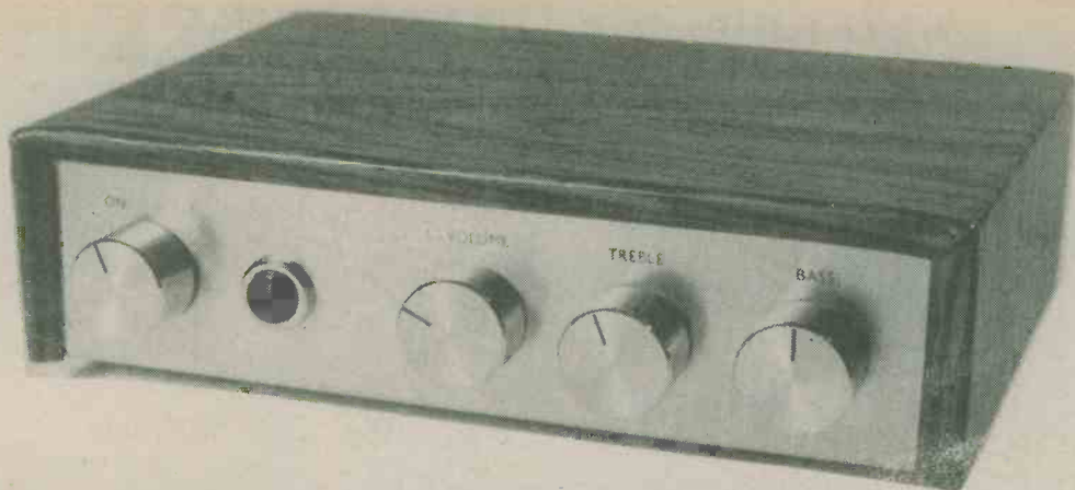
Front panel layout for the amplifier. On the left is the on-off switch with the neon pilot light to its immediate right. Next in order are the volume control and the treble tone control, with the bass tone control at extreme right
