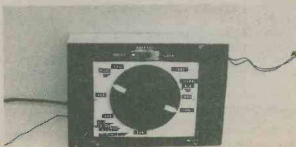
A large knob is required for VC1. This may be fitted with pointers and a tuning scale
