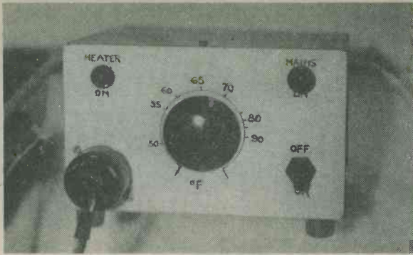
The temperature control unit. The large central knob sets up the temperature to which the propagator is taken
