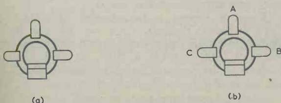
Fig. 3(a). The jack socket, as viewed from the rear (b). The tag letters, read in clockwise order, spell out the word "CAB"
