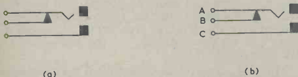
Fig. 2(a). Circuit symbol for the jack socket (b). The contacts may be identified by the letters A, B and C
