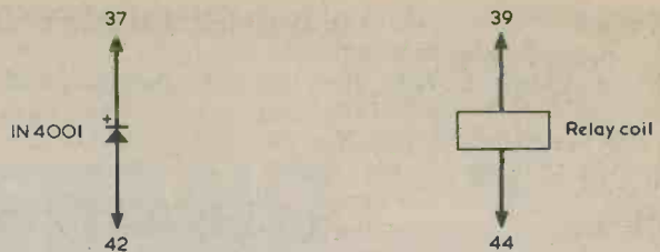
Fig. 2. A relay coil can be connected in place of PL1. It may have an operating current of 12 to 70mA and should energise reliably at 6 volts. Also required with the relay is a protective diode, which must be connected into circuit with correct polarity
