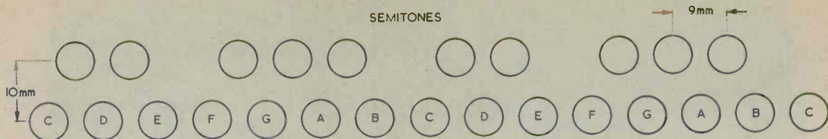
Fig. 2. The organ keyboard consists of 25 nickle plated screw heads laid out in the manner shown here
