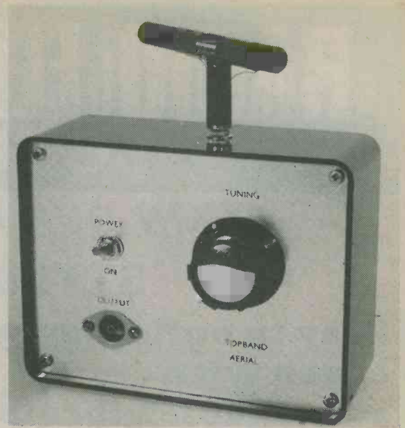
The Top Band active ferrite aerial unit. This incorporates a buffer amplifier to convert the high impedance signal voltages across the aerial coil to a low impedance suitable for coupling to a short wave receiver. The aerial above the case is free to be rotated
