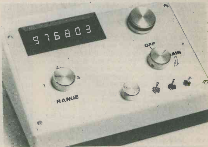
Framing the numeric display at the upper left edge of the panel is the new Vero rectangular display bezel. Simple to fit in place, the bezel not only covers unsightly tool marks but also gives an attractive frame and highlights the display
