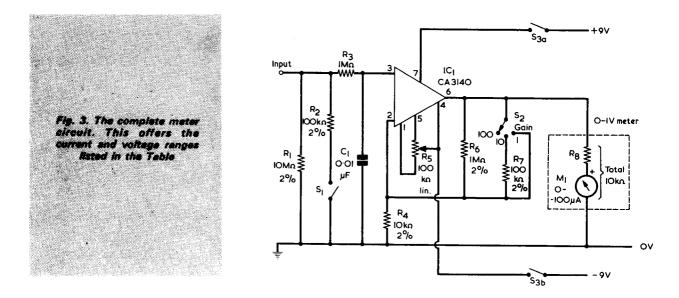
consist of employing a centre-zero  $100-0-100\mu A$  meter movement; the circuit could then measure input voltages and currents of either polarity.
