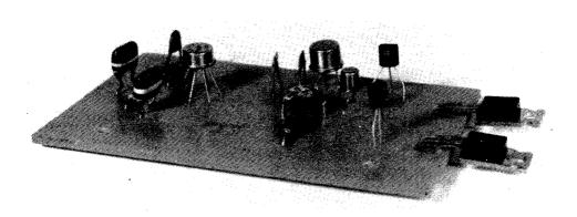
The d.c. coupled amplifier module. The two output transistors appear at the extreme right
