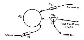
Fig. 6. Wiring details for the "S" meter circuit
