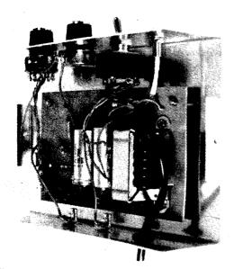
The printed board is spaced away from the bottom of the case to prevent short-circuits to its underside
