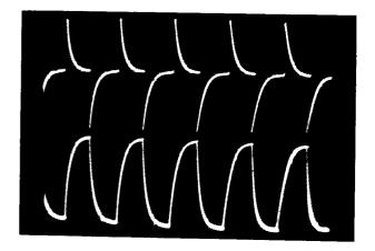
Waveforms at the inverting input (upper) and the output (lower) given with a low level 1kHz square wave input
