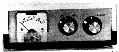
Front panel layout of the thermometer. The meter gives direct indications, in degrees Centigrade, of the temperature of the remote sensor
