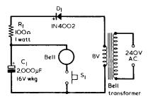
Fig. 2. Running costs are reduced to a negligible level if the single ping circuit is powered by a bell transformer.
