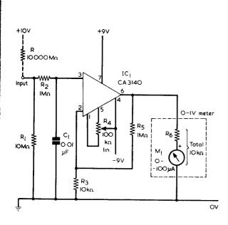
Fig. 2. Simple operational amplifier circuit capable of low current and voltage measurements
