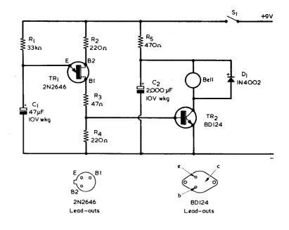
Fig. 3. A circuit which causes a series of pings to be sounded at approximately 3 second intervals
