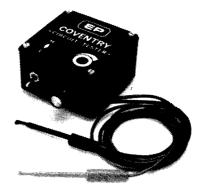
Circuit tester type CT.6, manufactured by Electronic Products, Coventry. This contains a miniature speaker which emits an audible tone when the test probes couple to a circuit path of less than a specified maximum resistance
