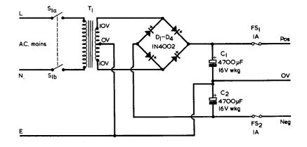
As shown, the power supply of Fig. 6 offers the positive and negative rails for the d.c. version of the
