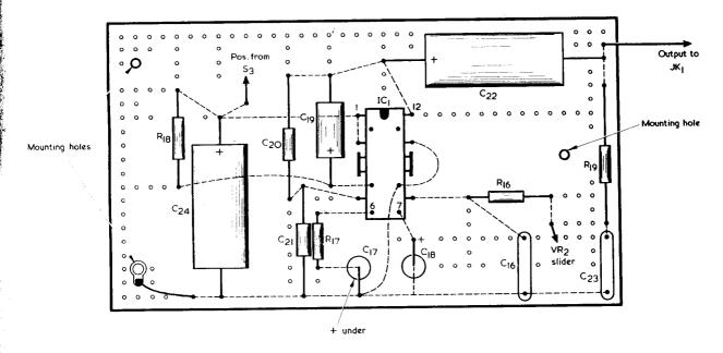
Fig. 8. The audio amplifier board is wired as shown here. Wiring under the board is reproduced in broken line
