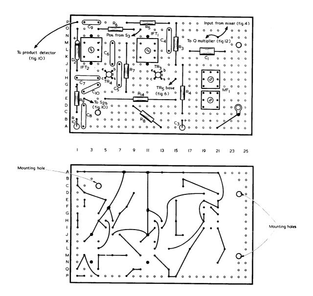
Fig. 5. The component and wiring sides of the i.f. amplifier
