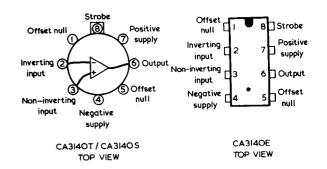
Fig. 1. Pin connections for three versions of the CA3140 RADIO AND ELECTRONICS CONSTRUCTOR
