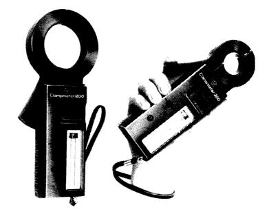
Two Avo instruments, the Clampmeter 1200 and the Clampmeter 300. The ends of the instruments are clamped over single conductors carrying high alternating currents to obtain current readings without the necessity of a direct connection
