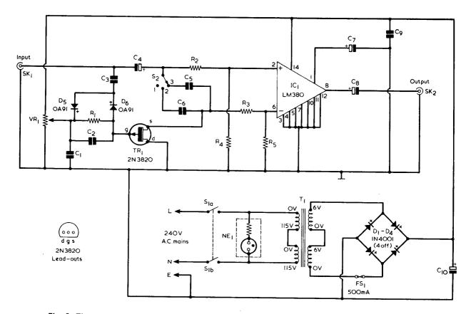
Fig. 2. The complete circuit of the noise reduction amplifier. The use of an integrated circuit audio amplifier considerably reduces complexity
