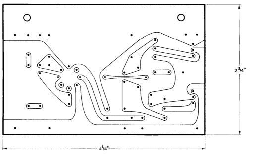
Fig. 5. The a.c. coupled amplifier is assembled on its printed board as shown here. Like Fig. 3, this is reproduced full size
