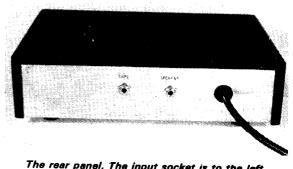
The rear panel. The input socket is to the left, with the output socket appearing between this and the mains lead
