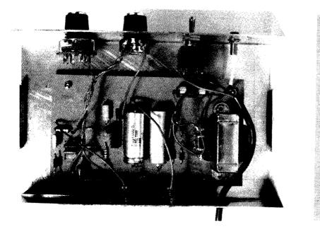
Looking inside the amplifier case. Wires from the printed board to the front panel components may, for nestness, be lightly twisted together as shown here
