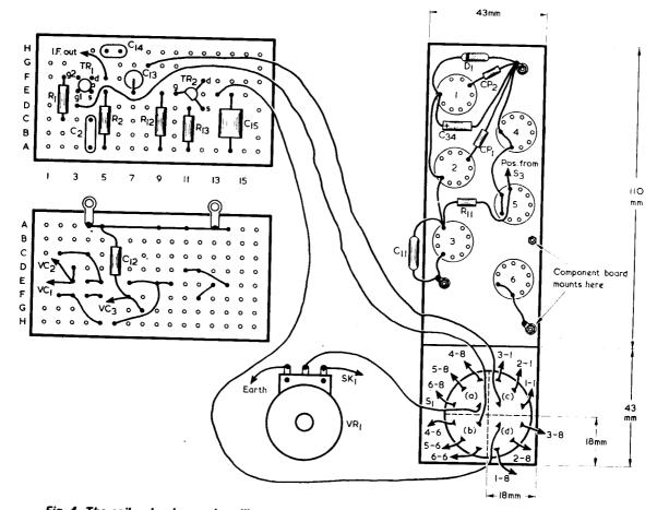
Fig. 4. The coilpack mixer and oscillator stages. Further details on these are given in the text. Pin 2 of coil 5 is used as an anchor tag
