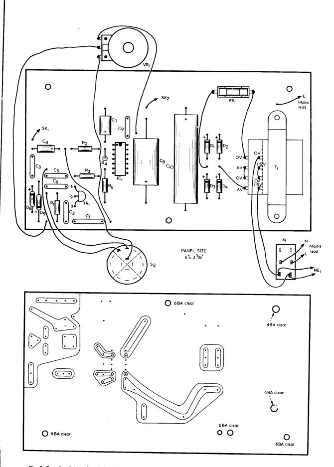
Fig. 3. Details of the printed circuit board, which is reproduced full size. The large copper area at chassis potential provides heatsinking for IC1
