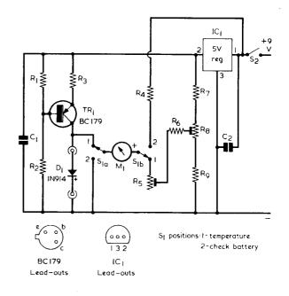
Fig. 2. The circuit of the remote read-out thermometer. In the lead-out inset for IC1 the leads are pointing at the reader
