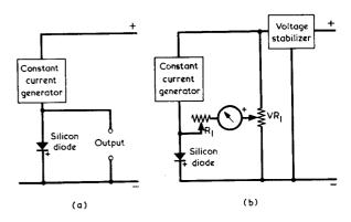
Fig. 1(a). In this circuit the voltage actoss the silicon diode varies in linear fashion with the diode temperature
