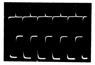
Waveforms with a high level 1kHz square wave input. Only supersonic harmonics are fed to the inverting input and the output shows little evidence of high frequency attenuation
