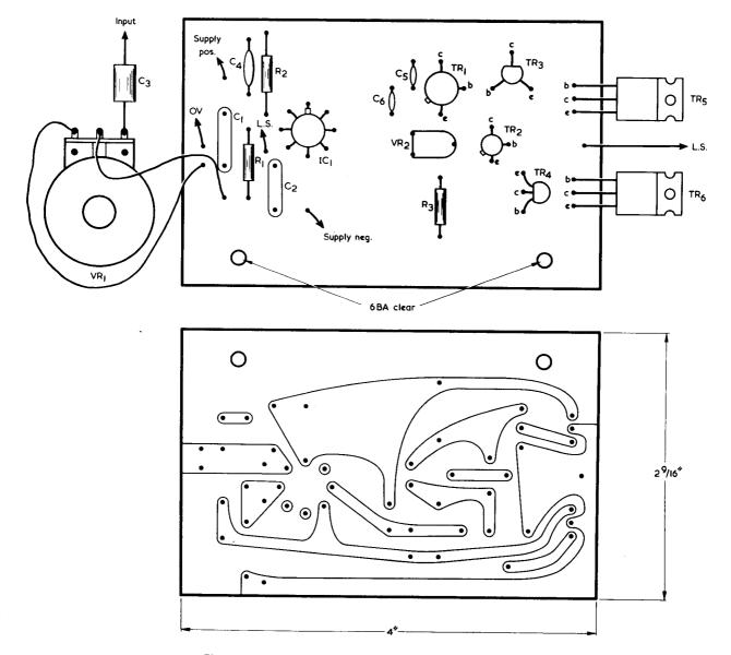
Fig. 3. The printed circuit layout for the d.c. coupled amplifier
