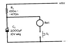
Fig. 1. A simple battery operated circuit. The bell gives a single ping when the push-button is pressed ed after operation of the bell the only current which flows is leakage current in this capacitor. With modern electrolytic capacitors this should be of the order of a few microamps only, or even less. The circuit functions with supply voltages down to some 6.5 volts, but the waiting time, as C1 charges after release of the push-button, becomes significantly longer at these low voltages.
