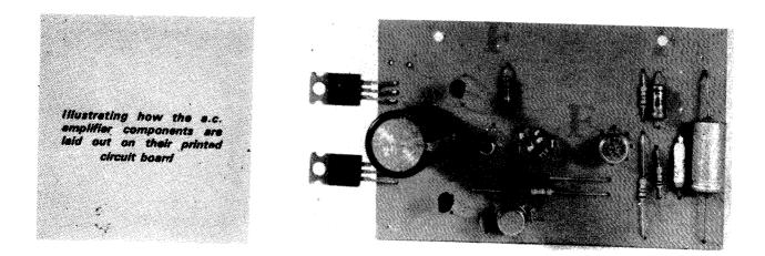
A suitable printed circuit board design for the a.c. version of the amplifier is reproduced actual size in Fig. 5. The construction and setting up of the circuit is the same as for the d.c. amplifier except that, due to the different layout, VR2 should be initially set fully clockwise if its slider is to be at the end of the track connecting to TR2 collector. It is then adjusted in an anticlockwise direction.
