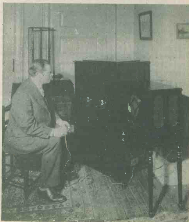
The first American home television reception took place in 1927 at the Schenectady residence of Dr. Ernst F. W. Alexanderson. The television screen is in the small square at eye level. A television system developed by Alexanderson and his co-workers transmitted pictures nationwide throughout 1928
