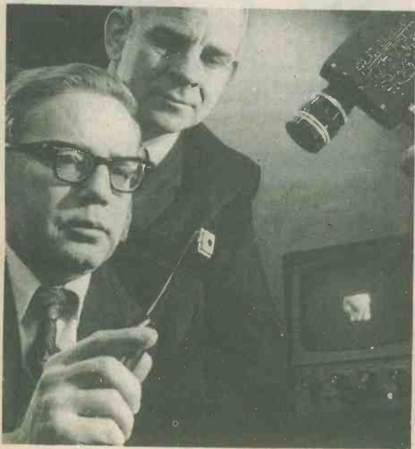
Gerald J. Michon holds a solid state imager in front of an experimental model of the newly developed General Electric solid state TV camera, causing its image to appear on the monitor screen. Watching is Hubert K. Burke who also worked on the camera. The imager replaces the bulky video tube currently used in conventional TV cameras and may lead to small inexpensive TV camera for home use.
