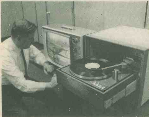
The Phonovid system in operation. Both the turntable and the television receiver are conventional, the information on the Videodisc being stored in an electronic memory which builds up a complete still picture in six seconds. A following picture is built up in the memory while the displayed picture is being shown. The disc also provides simultaneous high quality sound.
