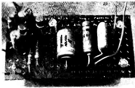
The Veroboard panel on which the circuitry around TR2 and TR3 is assembled
