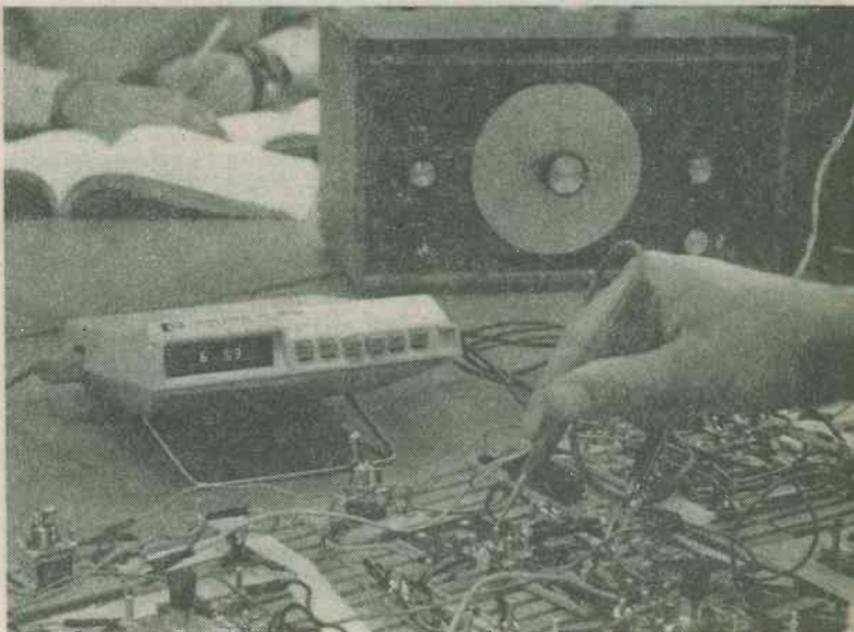
Sorting out the voltages in a complex experimental breadboard layout with the aid of the Hewlett-Packard digital multimeter
