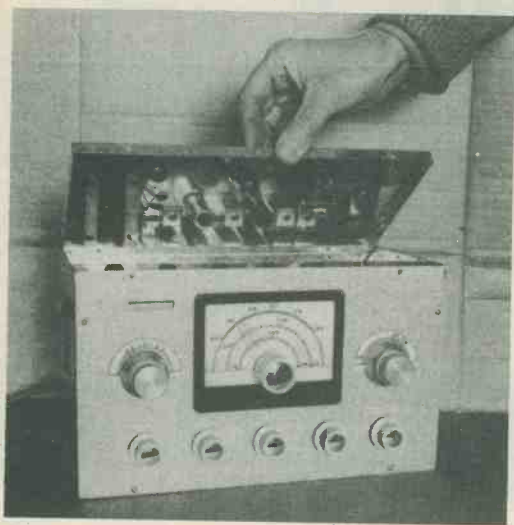
The inside of the receiver is reflected by the underside of the lid when this is raised
