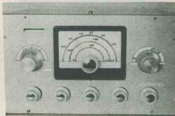
Front panel layout of the receiver. The tuning indicator is fitted behind the horizontal slot at the left of the central tuning drive
