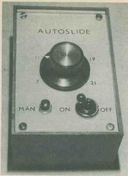
Another view of the completed timer unit
