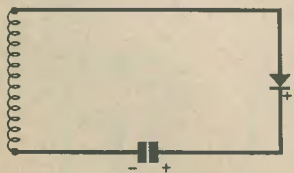
Fig. 6. The first bypass capacitor following an a.m. detector diode charges up with the polarity shown here, whereupon the diode is reverse biased between half-cycle tips
