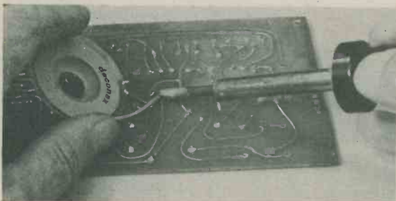
Deconex desoldering strip in use, assisting the removal of components from a p.c.b.
