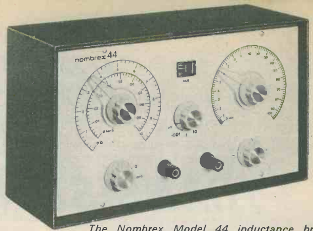
The Nombrex Model 44 inductance bridge, which is capable of measuring inductances from 1 \mu H to 100H. This incorporates two measuring processes, allowing readings to be taken with air-cored and iron-cored inductors
