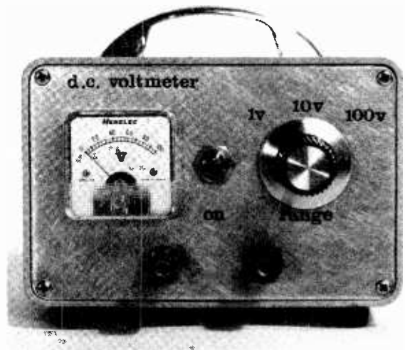
Another view of the front of the instrument. The prototype had three ranges, but further ranges can readily be added, as desired
