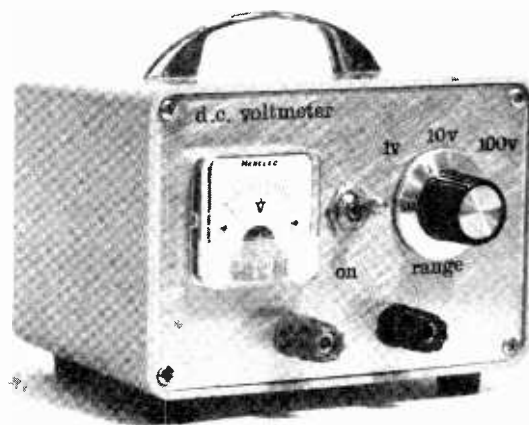
The complete voltmeter in its case. This measures 4 by 6 by 4in
