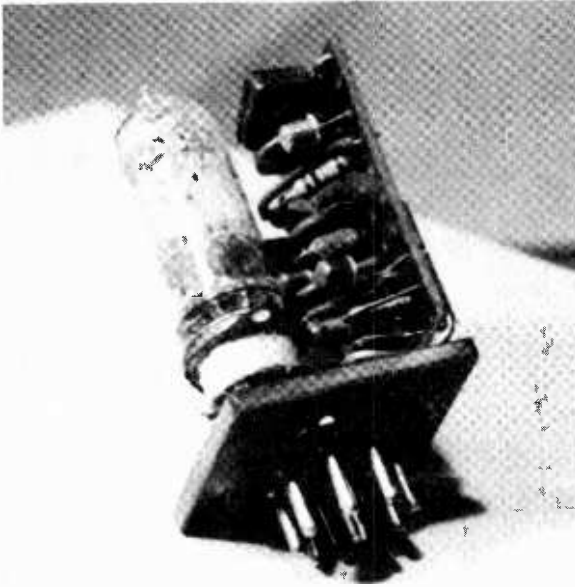
Side view of the completed marker unit, with the parts mounted on the octal plug
