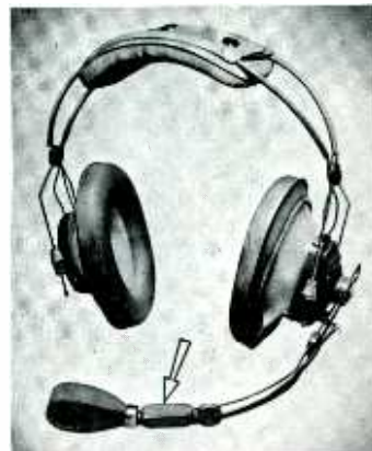
The micro-miniature pre-amplifier fitted on a Jetlite Headset
