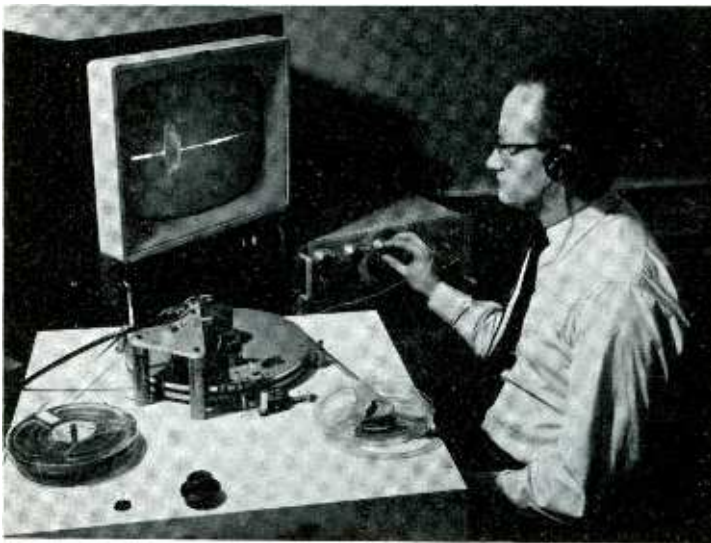
The rotating head system of the Speech Microscope, which replays repetitively the portion of stationary tape which is wrapped around part of the periphery of the rotating disc. The equipment can be used to study the duration of sounds necessary for correct speech recognition
