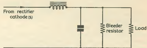
Fig. 275. Adding a bleeder resistor across the output from a choke input filter
