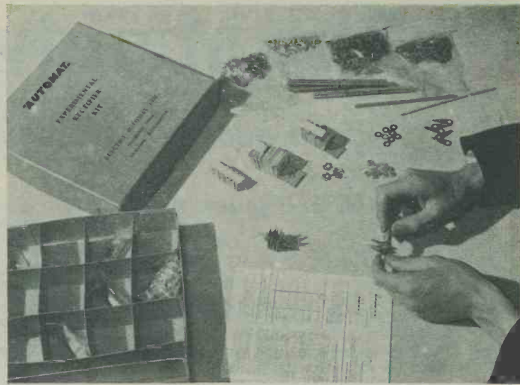
Do-it-yourself rectifier assembly. The newly introduced Electro Automat rectifier kit allows the assembly of rectifier stacks to meet exact circuit requirements
