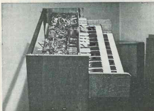
The stop tray viewed from the side. The pre-amplifiers are mounted at the rear
