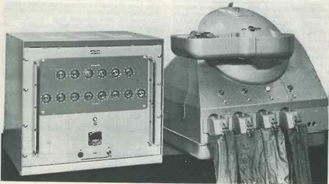
APTEC 100 coin counting system in use with M.1000 sorting and bagging machine
