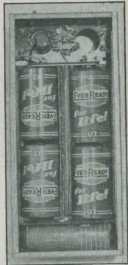
Showing arrangement of batteries within the case
