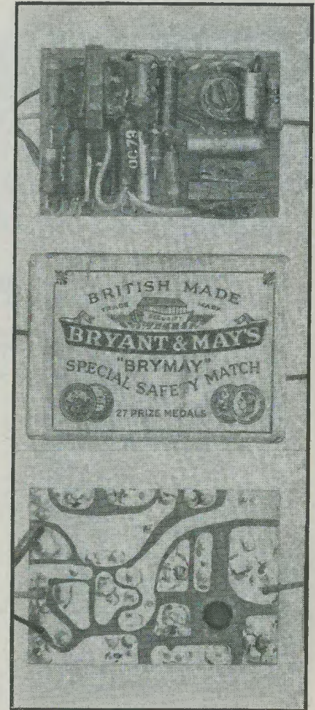
Fig. 1. 3-transistor receiver on printed panel
