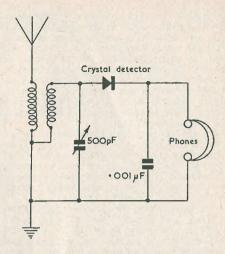
FIG.2. THE CRYSTAL DETECTOR
