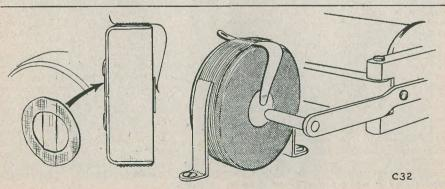
Fig. 32. Construction of pneumatic delay.
