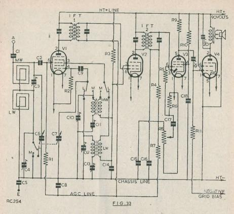
Circuit of a receiver suitable for use with the power supply shown in Fig. 32
