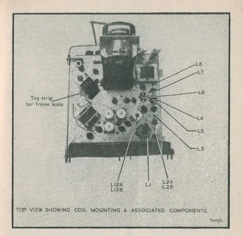
is placed between the coils and focus unit to prevent shorting the deflection connections. The Line-output transformer may now be installed. This is drilled especially for small Parker-Kalon self-threading screws. The EHT rectifier is carefully soldered into position as shown in the sketch. The greatest consideration must be given to the soldering—sharp points should be avoided. The EHT lead is attached as shown.
