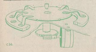
Fig. 36. Construction of a motordriven coding switch. Keying brushes are not shown
