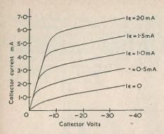
FIG. 3. Static characteristics of typical point contact RC270 transistor
