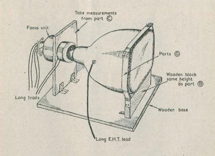
TEMPORARY MOUNTING OF TUBE ASSEMBLY
