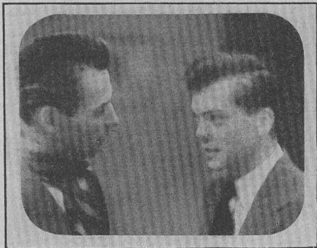
Fig. 2: Loss of interlace. The raster lines show clearly when one frame scan is superimposed on the next, as here.
