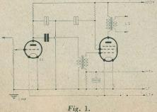
may be likened to reaction in the opposite phase. i.e., whereas reaction is positive feed-back which increases gain at certain frequencies, this type of feed-back is negative and decreases gain and so tends to flatten the response curve of the output stage.
