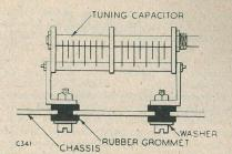
Fig. 15. A vibration-proof mounting for a tuning capacitor.
