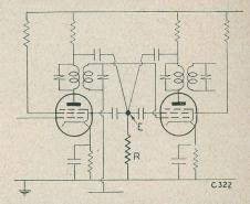
Fig. 10(a). Indicating how a badly connected earthing return, if for several circuits, may actually assist feed-back. The feedback voltages, at different stages of amplification, are built up across the resistance "R," which represents the resistance of the joint. (E is the earth tag with high resistance ioint.)
