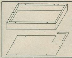
In considering this problem I have devised, what, for the want of a better name, I have called the "Free Deck" Chassis. It has a steel frame for strength and rigidity and an aluminium mounting area for easy workability.
