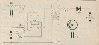
oscillator anodes needs around 90 volts this series resistor must be removed. This is usually an easy matter. The neon should be stood in methylated spirits for a while. The base can then be removed and the series resistor taken out. Plaster-of-Paris can then be used to cement the neon and base together again.
