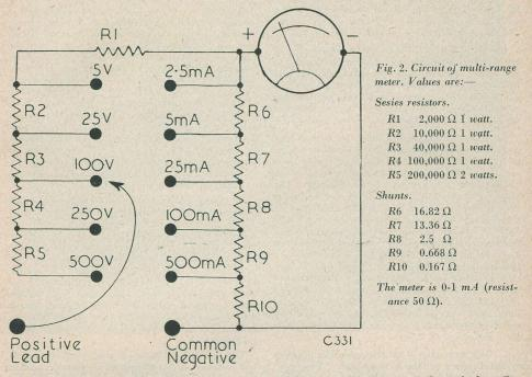
of that stated. If trouble is experienced in obtaining a certain resistance value it may generally be made up from a number of components. However, failing this it is possible to slightly increase the resistance of carbon resistors by reducing their cross-sectional area. This may be achieved by carefully filing a flat on the body of the component, the increase in resistance will be governed by the depth and length of the portion which is removed.
