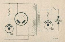
Fig. 5. Neons may be installed as voltage indicators in the power pack. Series resistors may be from 1-5  $M\Omega$  dependant on the current taken and consequent voltage drop.
