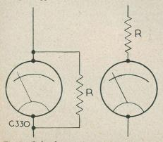
Fig. 1. Left-shunt resister to increase current range. Right-series resister to increase voltage range.
