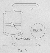
This can be done electrically too. If the pump is replaced by an electric battery the two arms are replaced by upper wires, and connected to the battery, as in Fig. 1(b) with a current meter needle to deflect, owing to current flowing in the centre limb of the network. Taking this idea further, we can substitute resistance for the wires as shown in Fig. 1(c) and for a null reading on the meter
