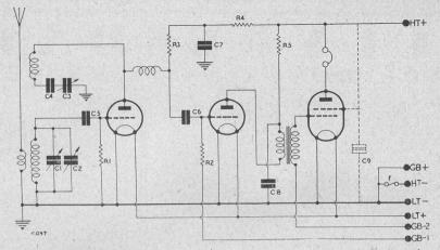
The dotted lines shown in output stage apply only if a pentode output valve is used.
