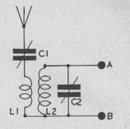
Fig. 2. L2 and L2 are standard SW coils to cover 6–9 Mcs. C1 is 100  $\mu\mu$ F and C2 is 160  $\mu\mu$ F. Points A and B are connected to RF pin on receiver and chassis respectively.
