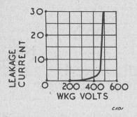
Fig. 2. Leakage characteristics of a typical  $16 \mu F$ , 400 V, wet electrolytic capacitor.
