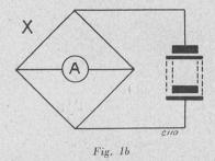
100 to 1, or 1,000 to 1 is used, and R4 is calibrated accurately. R3 is connected to the bridge by means of test terminals, and the bridge is balanced, that is the setting is adjusted until no reading is obtained on the meter.
