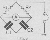
previously is admirable. Detection of null point is achieved by using headphones. Due to stray capacitance effects in the oscillator, the sound never actually disappears, but the minimum point is easily distinguished.
