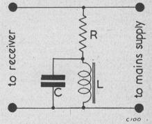
Fig. 3. Shunt connection for mains energised speaker field.
