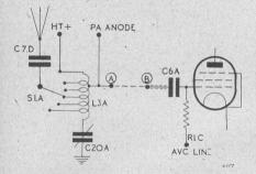
Fig. 1. (left) the TX PA circuit and (right) the RX RF stage. "A" goes to the RF socket on TX panel and "B" goes to RF pin on RX 5-pin plug. In the 18 Set, the circuits are permanently connected as shown by the dotted lines from A—B.
