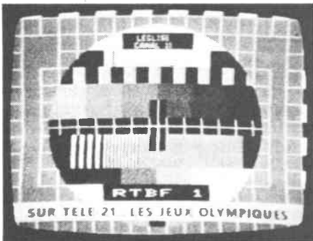
Fig 1: PM5544 test card received from Belgium on E11 during the 1988 Olympic Games
