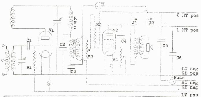
dials are Admiralty precision from Messrs J.B. Service and were easily adapted to operate the variable condensers through flexible couplers. The very low capacity variable condensers are from TR9 and No 21 receivers, the former being used for grid circuit tuning. These twin ganged condensers are not used in a normal manner -- the 6-pin coil is virtually a 4-pin across ONE section of a condenser, links being used on the additional pins to bring in the OTHER section of the condenser in
