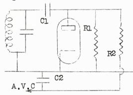
In this figure Rl is the diode load and R2, C2 are the smoothing. Now the great snag here is the damping imposed on the tuned circuit (which is usually already damped by the detector anyway). This damping is equivalent to shunting a resistor, value Rl/3 across the tuned circuit.
