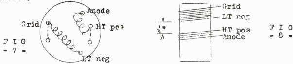
AMATRUR BAND COIL DATA, found in the prototype to be satisfactory without adjustment. The former diameter is  $1\frac{1}{2}$ " and the tuning capacity .00005 uF. Enchelled wire is used for the coils which are spaced  $\frac{1}{2}$ " except where indicated.
