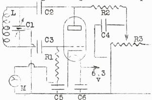
Cl is a 25 x 25 pF midget splitstator condenser. C4, 5 and 6 are .0005 uF midget micas. C2 is 50 pF and C3 is 10/30 pF, also midget micas. R1 and R2 are 20 K and R3 is a 100 K pot. The meter is a 0/500 uA moving coil. The valve is a 6J5. L is a 3 turn coil of 14 swg enamelled, the windings spaced to  $\frac{3}{8}$ " inch long. The coil is mounted out from one end of the chassis on  $2\frac{1}{2}$ " long supporting wires. It is important that the connections from C1 to the valve should be as
