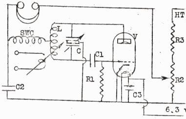
This is a normal superregen receiver. Any type of <u>self-oscillating</u> super-regen Rx can be used. The only thing to note is that the condenser must be placed so that the coil L can easily be soldered on and off.All grid and anode leads must be kept to the absolute minimum length. All earth leads should come to a common tag. A 7193 gives the best layout.
