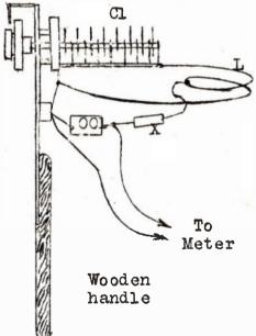
Values for the wavemeter are:- L, 2 turns, 16 swg enamelled,  $\frac{7}{8}$ " diameter, spaced 3/16" batween turns, centre tapped. Cl, 100 pF midget variable. C2, .001 uF midget mica. X, germanium diode. The meter should be 0-500 uA, and a small epicyclic drive (5:2.) will be required for Cl. The coil and condensars should be earthed to a common tag. Approximate coverage is 60 - 150 Me/s.
