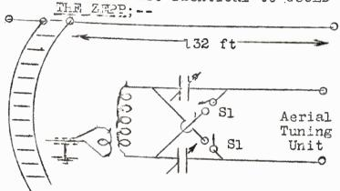
The feeders are 44 ft in length and the spreaders are 10" AM ceramic type. Sl is a parallel/ceries switch. All wire is heavy gauge, 14 or 12 swg cadmium copper.
