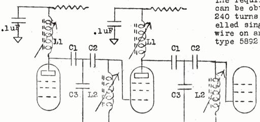
The required inductance can be obtained by winding 240 turns of 36 swg enamelled single silk covered wire on an Aladdin former type 5892 which is 11/32"
