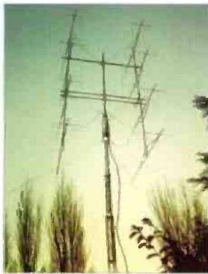
Fig. 1: David Johnson G4DHF's eight 11-element Yagis - over 90 QSOs were made in a three hour period!
